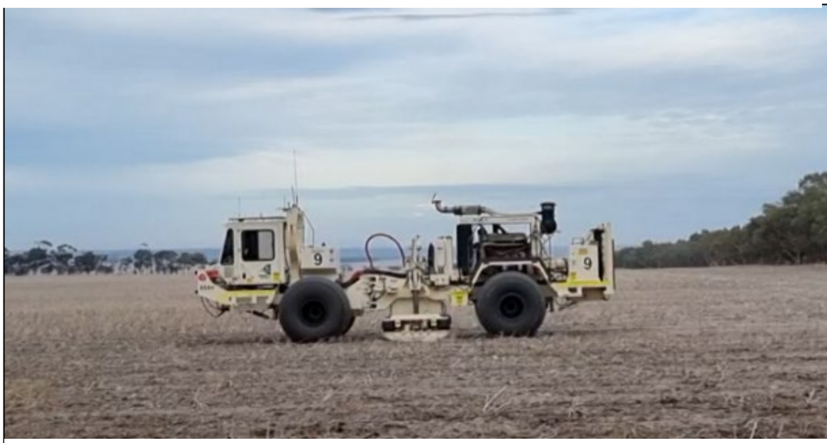
Figure 8: Bookara 3D Seismic Vibroseis seismic acquisition vehicle near Mt Horner
