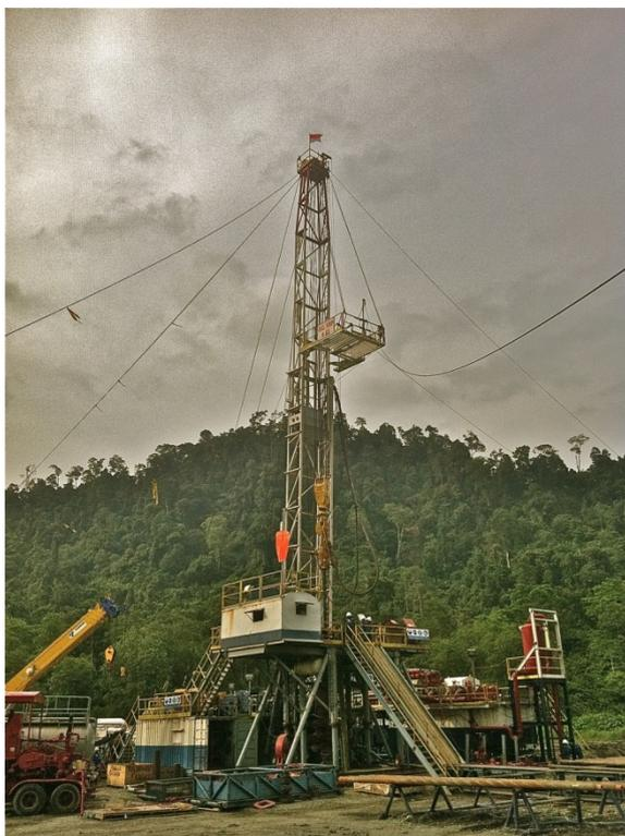
As at 11:00 Jakarta time two cement plugs have been drilled out of the Pase A-2 well to a depth of 9,025 feet measured depth. Preparations are continuing to drill out the two remaining plugs.
